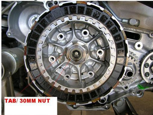
3. Remove clutch plates and inner hub.
