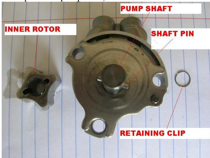
The bushing w/ o-ring, inner rotor, shaft pin, and new retaining clip (new clip provided with kit) must be re-installed on new oil pump before re-assembly.
