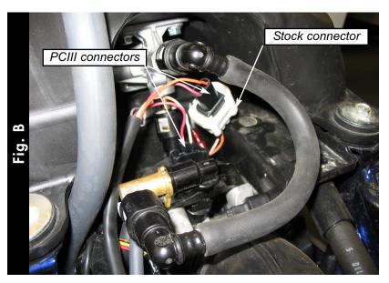
Plug the connectors from the PCIII inline of the stock wiring harness and fuel injector (Fig. B).
