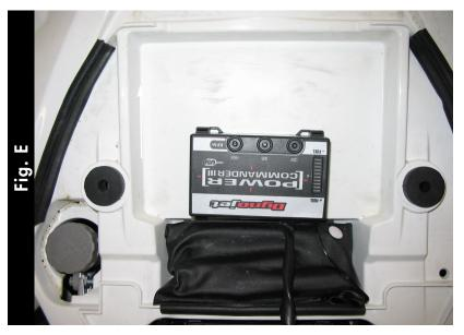
Install the PCIII to the rear fender as shown in Fig. E. Position the PCIII so it does not interfere with the foam pads on the bottom of the seat.
