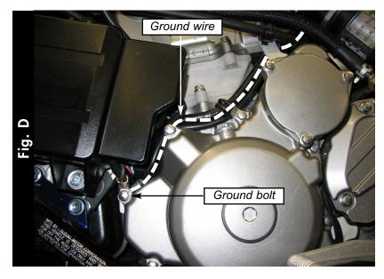
10 Attach the ground wire from the PCIII to the common ground on the left hand side of the engine (Fig. D).
