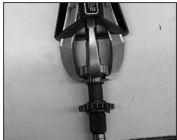
17. Remove bearing from other end of input shaft. Remove two snap rings and gear.
