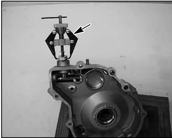
13. Remove snap ring and washer. Pull down and rotate shift fork shaft back and forth to remove.
