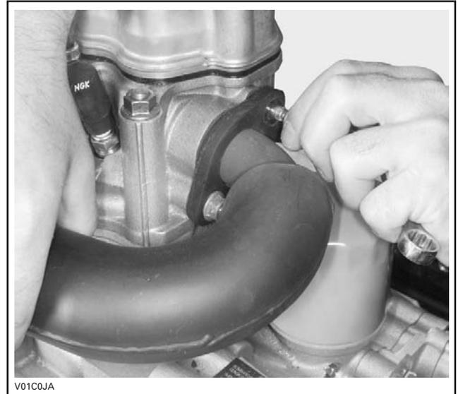
Remove screw from exhaust pipe bracket no. 16.
