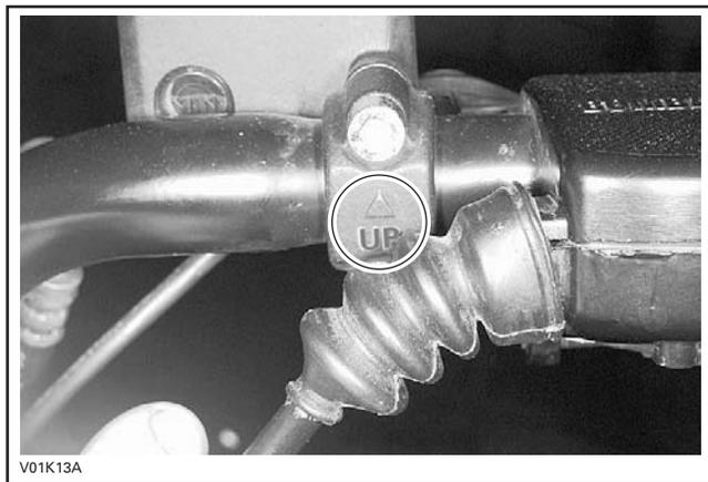
Connect brake hose to master cylinder with bolt and new sealing washers.
