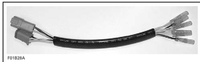
3. Connect one of the multimeter leads to the WHITE/YELLOW wire of the 6-pin magneto harness adapter.
