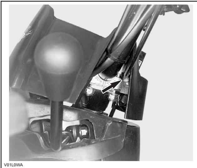
Remove ignition switch and choke lever.
